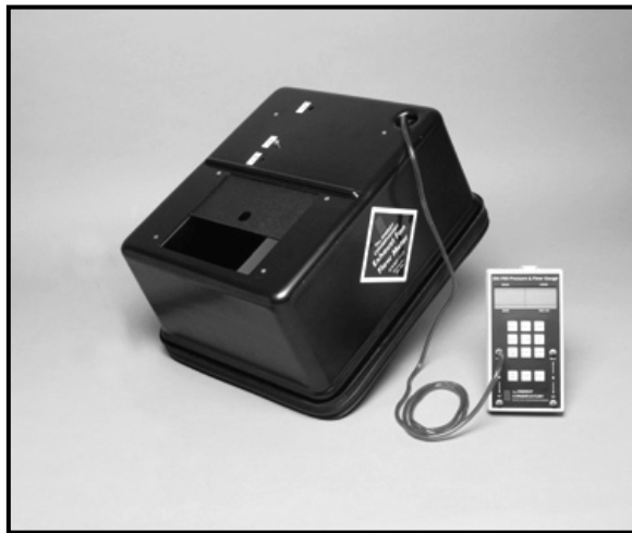
Exhaust Fan Flow Meter with DG-700 Pressure Gauge
