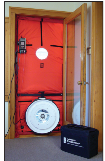
The Minneapolis Blower Door™ is used to measure the airtightness of buildings.
