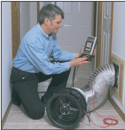
The Minneapolis Duct Blaster® is used to measure the airtightness of duct work.
