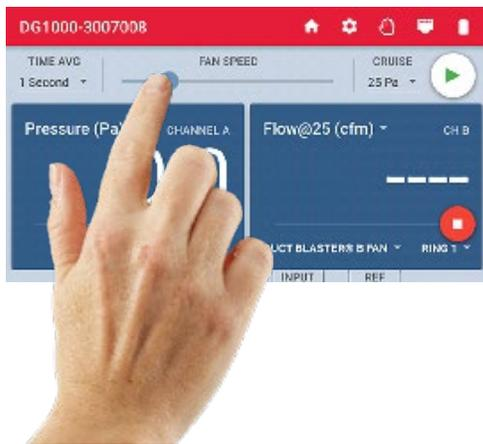
Touch and slide the dot on the fan speed slider in the Gauge app to adjust the fan speed using the DG-1000. As the fan speed increases, the duct pressure displayed on Channel A should also increase. Continue to increase the fan speed until the duct pressure shown on Channel A is between 20 and 30 Pa.
