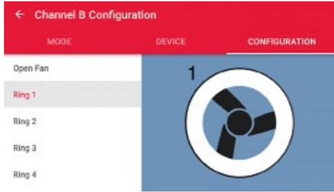
4. Install the flow ring which best matches the needed fan flow (see table below) and then select the same ring in the Configuration menu.
