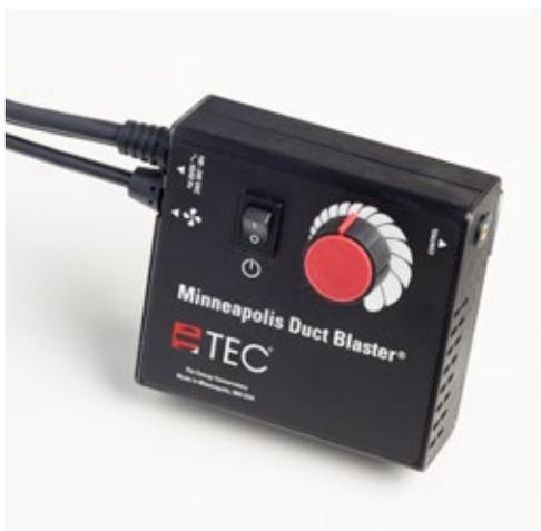
Gradually increase the fan speed by slowly turning the fan controller clockwise. As the fan speed increases, the duct pressure displayed on Channel A should also increase. Continue to increase the fan speed until the pressure shown on Channel A is between 20 and 30 Pa.
