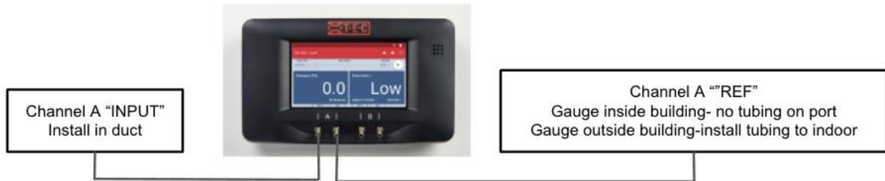
Figure 5: Connecting the Static Pressure Probe to a DG-1000
