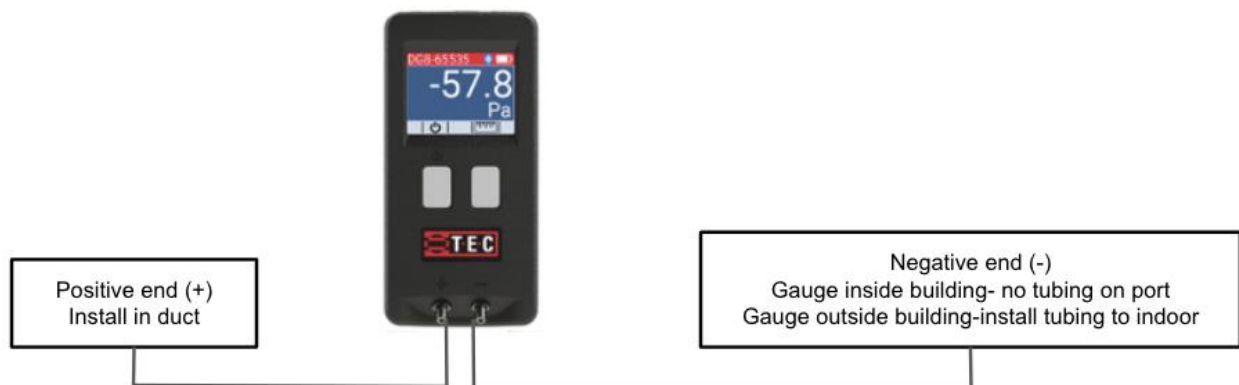
Figure 6: Connecting the Static Pressure Probe to a DG-8
