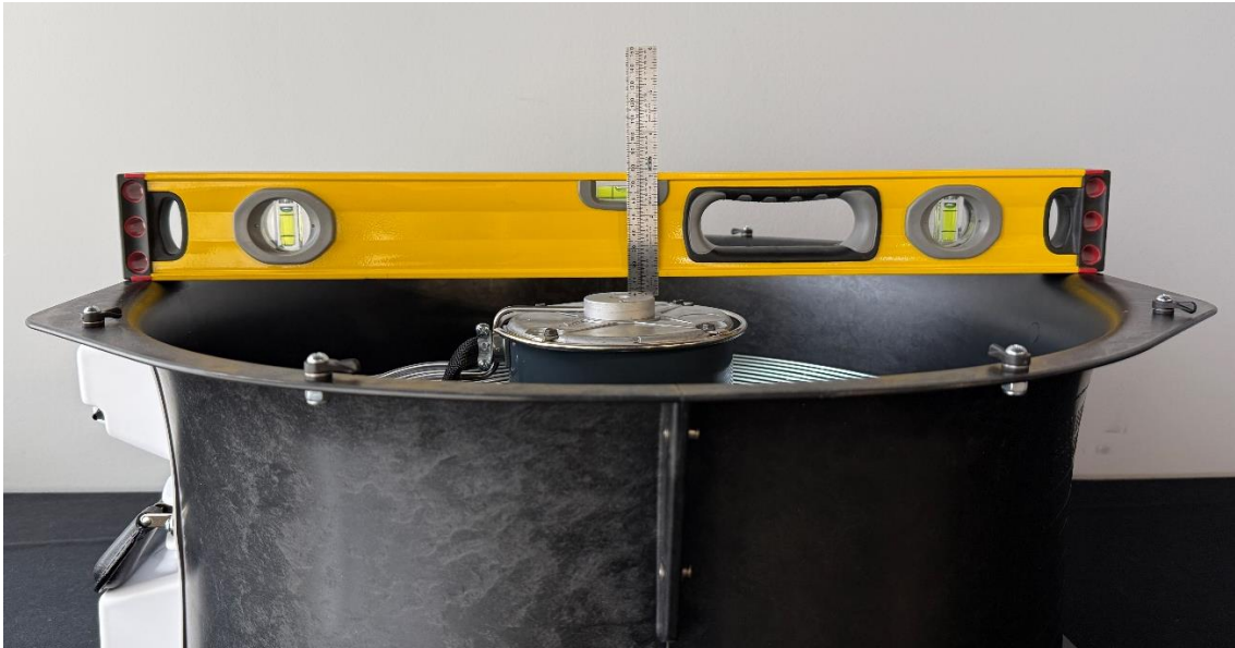
A straightedge across the fan housing with a ruler to measure the gap.
